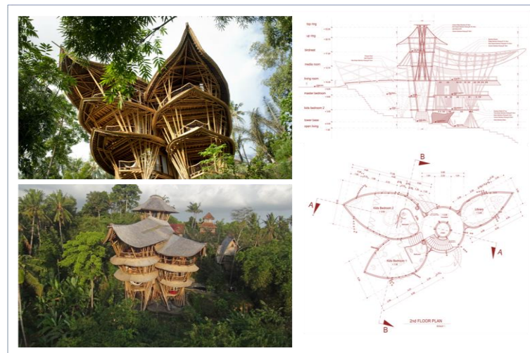
Fig. 2: Bamboo openwork house Sharma Springs (Bali, Indonesia, author: Elora Hardy, design bureau IBUKU, 2012) Source: ibuku.com.
